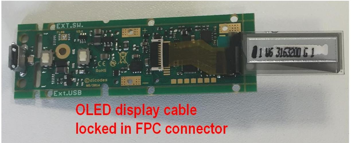
Now the cable is clamped and contacted.
