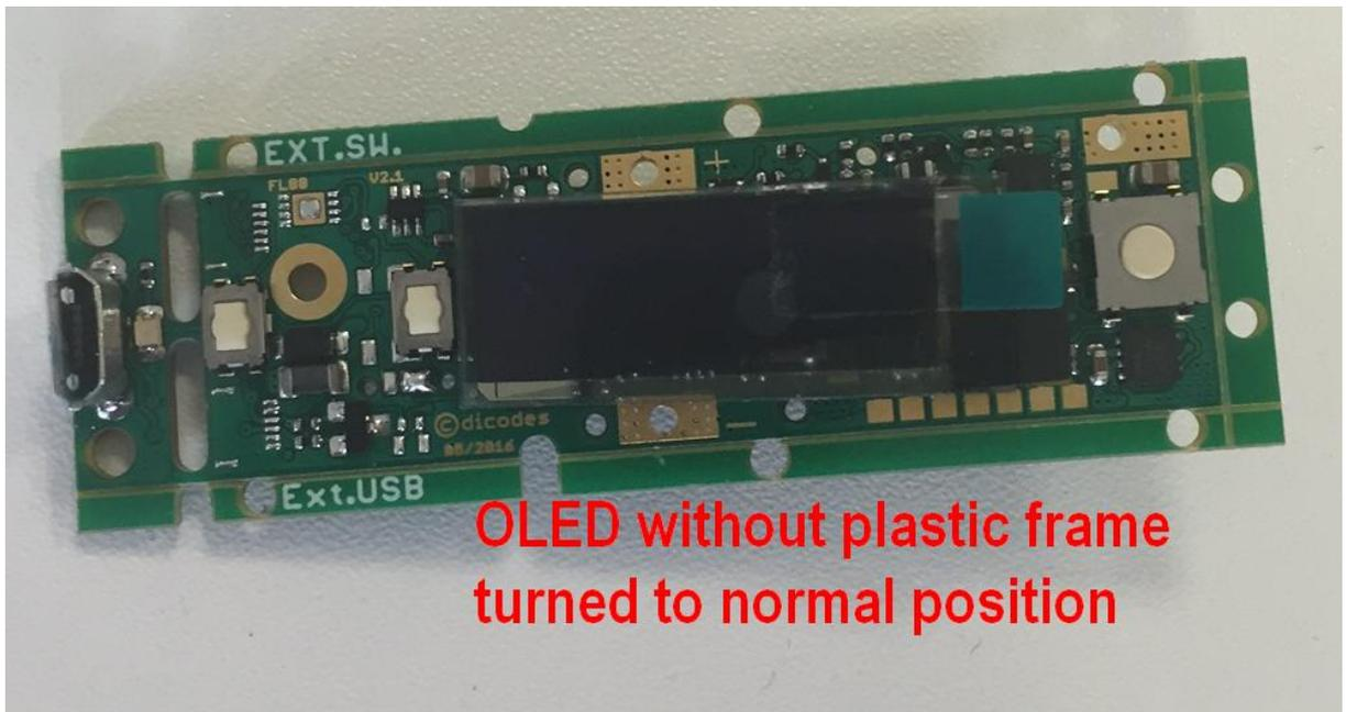
When the user wants to place the display somewhere else in the box/application, instead of plugging the OLED directly to the onboard FPC, a standard 12pin 0.5mm pitch FFC cable can be connected to the board which is then connected to a display carrier board at the other end.
