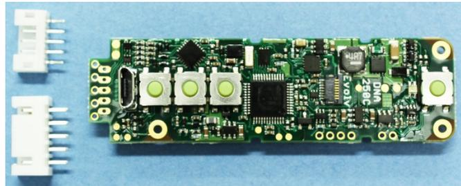
**Step 2:** The balance connectors are inserted in the appropriate holes on the back side of the board opposite the buttons and soldered in place. PH connectors will fit the row closest to the USB connection and XH series connectors will fit the row furthest from the USB connection.
