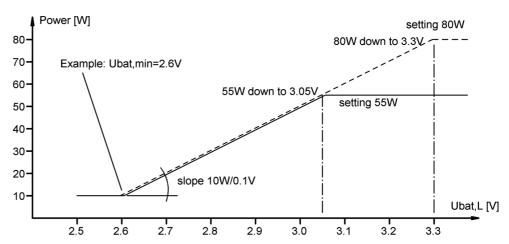
At UBatMin+ 0.7V a power reduction is activated depending on the actual power setting. The reduction starts when the power selected hits the slope from Ubat,min@10W to Ubat,min+0.7V@80W as show in the diagram above.
