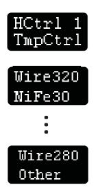
In this mode the mod will regulate the temperature of the coil to the pre-set value, except the power setting is too low to achieve the temperature. So please note to adjust the power setting to a value high enough, if you choose temperature controlled vaping. Otherwise the temperature regulation changes to a temperature limitation mode.
