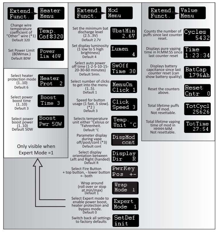
(\*1) The temperature coefficient selects the type of wire material in the range 050 to 650: When TC-mode is selected (Main menu HCtrl=1), the user must select the wire type to be NiFe30 (320, dicodes wire), Ni200 (620), Titanium (350), SS304 (105, V2A), SS316 (88), SS316L (92), NiFe48 (480) or "Other". The value for "Other" is adjusted here. Value to select = Literature-value\*10E5 K. Example: Ni 6.2E-3\*1/K \* 10E5\*K => 620
